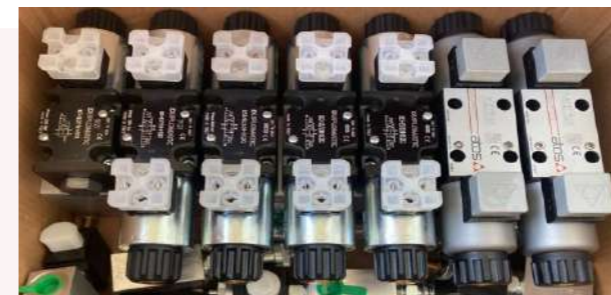
Figure 7 Electro-hydraulic unit with solenoid valves
