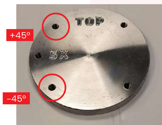
Figure 30 Indication on 45^\circ and 135^\circ angle counter-plate
